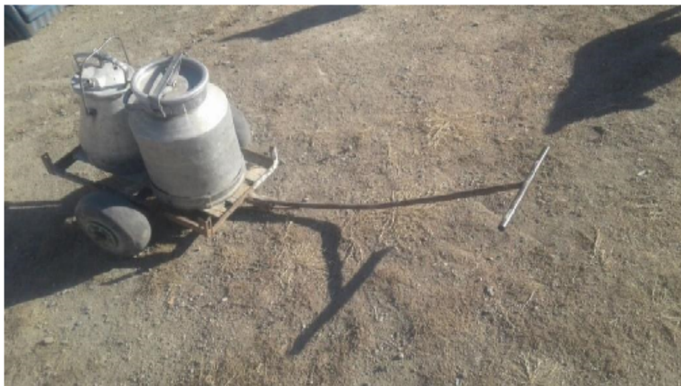
Figure 19 – A device for self-delivery of water to the house
